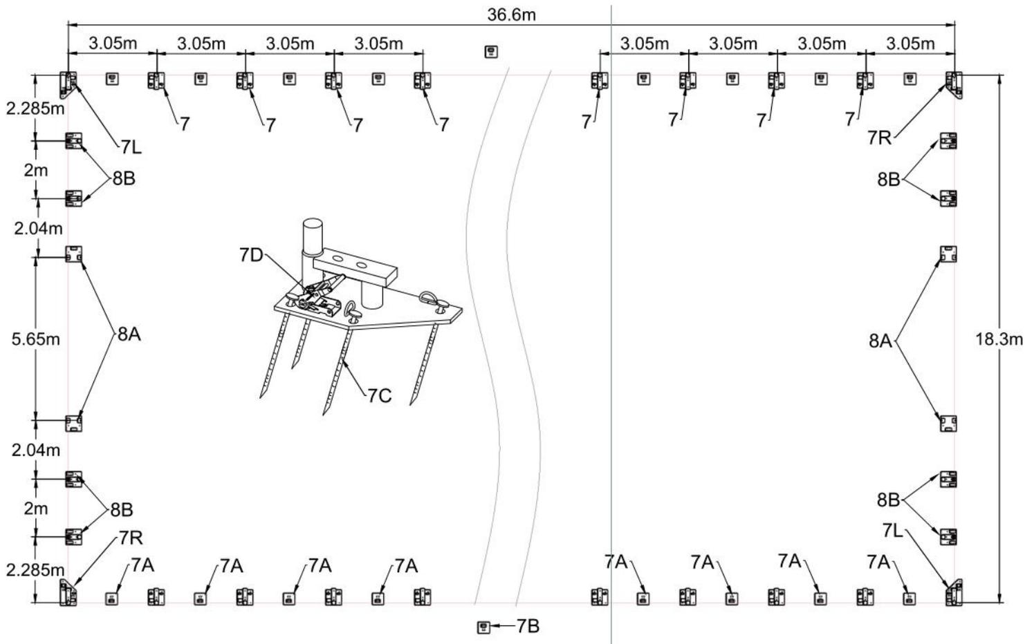
**Figure 2 Foundation placement**
