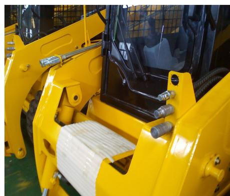
**Note: Ensure that the quick connector is fully engaged. If the quick connector cannot be fully engaged, please check whether the size and type of the connector are the same. Before making connections, thoroughly clean the quick connectors. Dust can quickly damage the system.**
