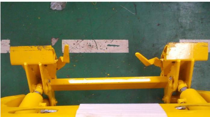
Drive the loader forward until the upper edge of the quick-change rack is completely on the upper flange of the quick-change device
