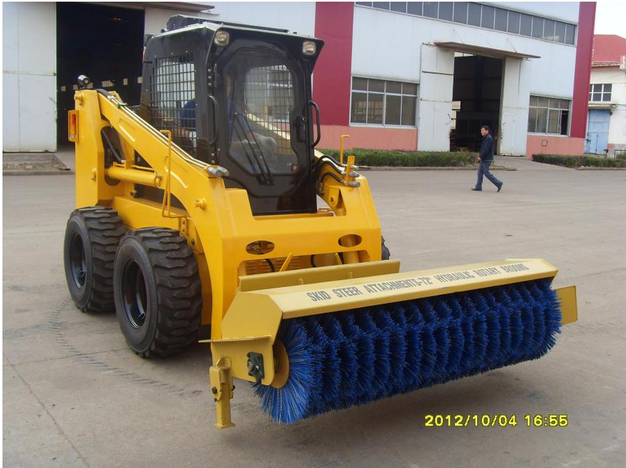
5. It is possible to adjust the left and right angle of the oblique cleaning machine to the rightmost deflection operation.
