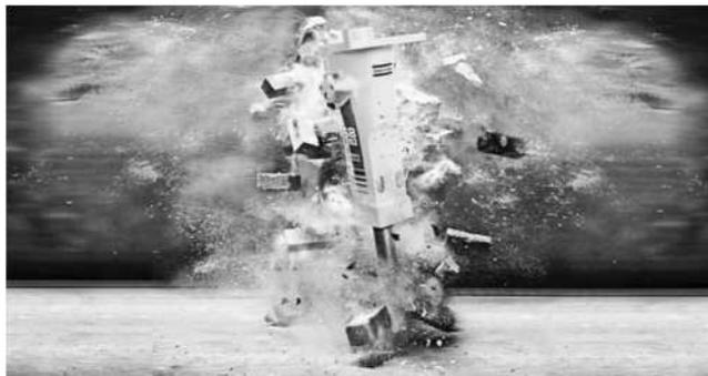
The hammer head shall be perpendicular to the working surface for breaking operation.
