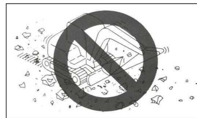
When the mini-excavator walks on the riverbed or where there are a lot of pebbles, it may cause the stones to get stuck in the caterpillar band and damage the caterpillar band, or make the caterpillar band fall off.
