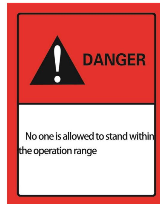
8. Stay away from the excavation area: this sign is located on both sides of the bucket arm.
