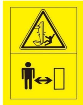
9. Hydraulic tank sign: this sign is located on the housing at the hydraulic oil tank.
