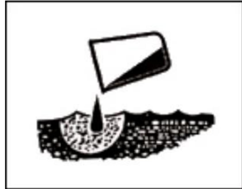
1. Ensure that the waste oil discharged from the mini-excavator is collected in a container. Improper treatment of waste oil will cause harm to the environment.
