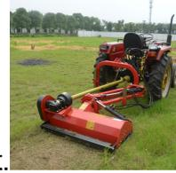
The picture shows the position of the machine during transport.
